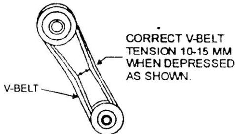
Figure 2. V-Belt Tension
