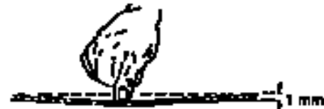
Fig. 1: Adjusting blade tension
